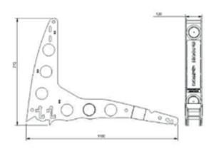
They are made of 2 steel sheets (thickness 8 mm / 0.31 in) connected with struts (thickness 8 mm).
