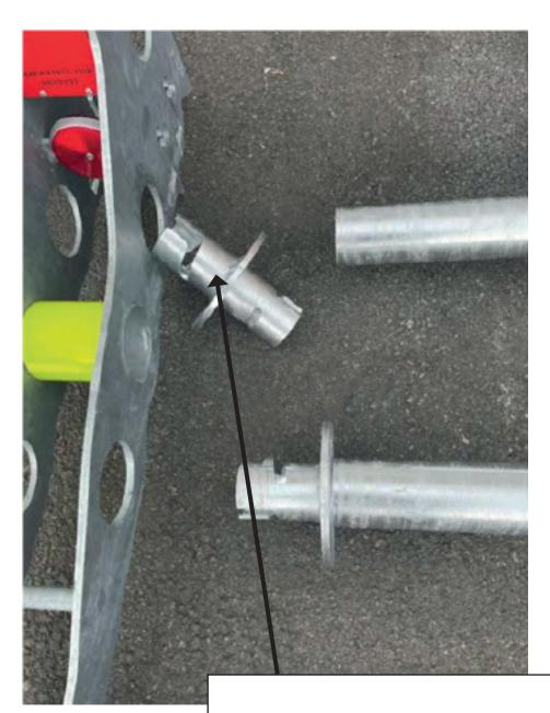
Warning: while screwing the plug the weld seam side should be on the block (it will be helpful for dismounting)
