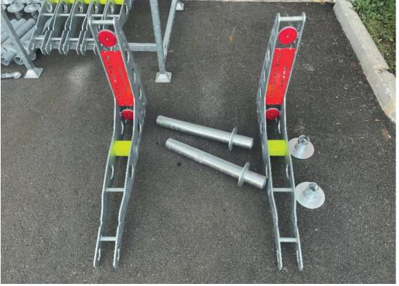
3. Setup 2 short start male tubes left side inside first block, then screw the plugs and connecting tubes in hole 1 and 3. (all these operations only by hand, no tools required)
